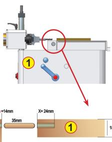
Turret Vitap with 6 different positions plus device to automatically change the vertical horizontal depth (-10 mm in vertical) to avoid the chipping of the panel
